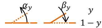
Figure 15. Ion channel gating kinetics. y is the fraction of gates in the open state. \alpha_y and \beta_y are the rate constants for opening and closing, respectively.
